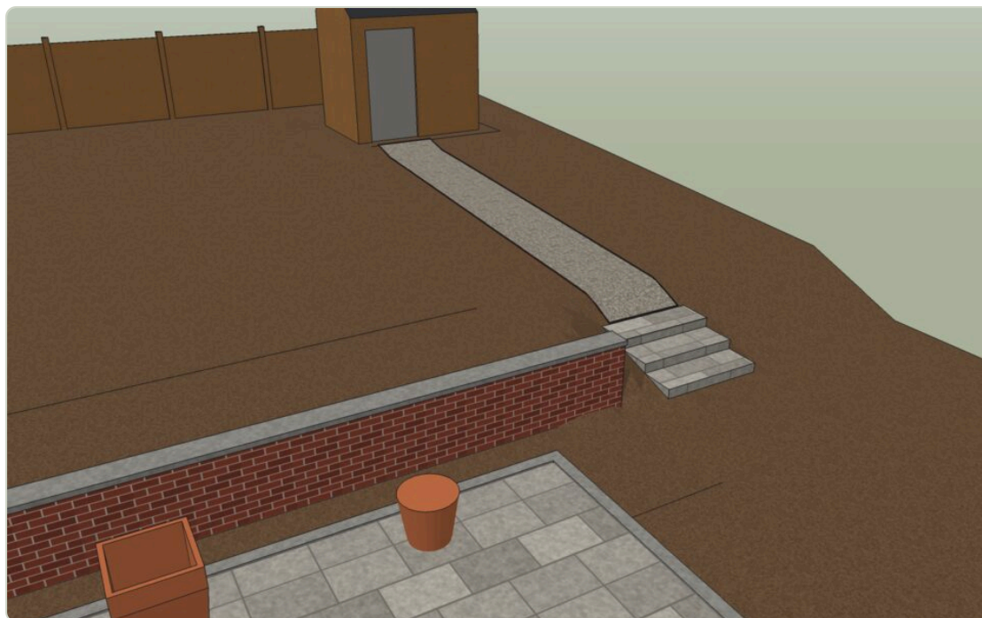
Figure 9.2 The patio with its kerb, the brick retaining wall with its cap, three steps and the gravel path to the shed.
